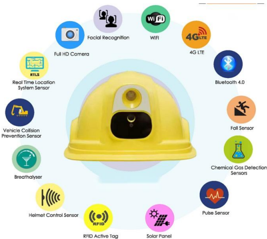
Figure 5. Smart helmet functions (Ouxiang International Limited, 2025)
